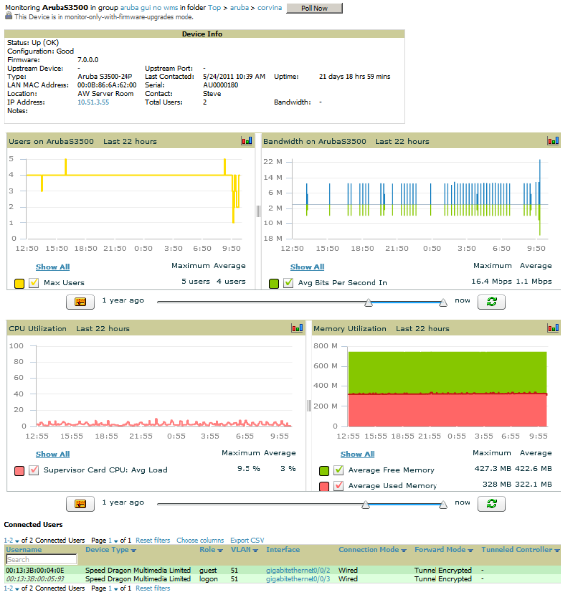
Figure 90 APs/Devices > Monitor Page for a Switch
